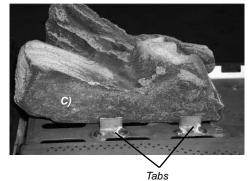
6) Take the embers and place on the burner in the space between the 2 front logs. Do not put embers on the burner in the area between the front logs and the rear log. See photo below.
